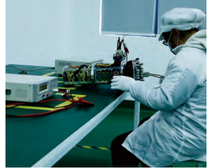
High Voltage Insulation Test
