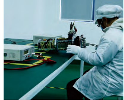
High Voltage Insulation Test
